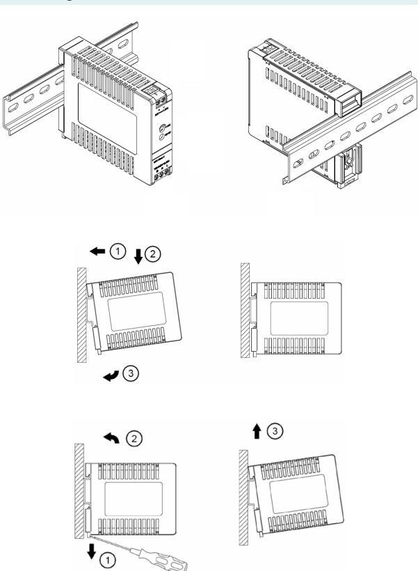
The power supply unit is snapped into place using a snap-on mounting. Several units can be easily connected in a row thanks to the optimized heat dissipation.
